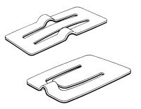
• Thermostat with snap action bimetal
